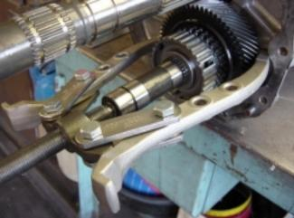
The brand is not important, but the reach is. You will need a 6-1/2" reach puller to reach behind the fifth drive gear, as shown...]. Carefully place the arms behind the gear (to avoid chipping the teeth), and turn the screw to pull both the gear and synchro hub off of the cluster gear. While it would be nice to pull the hub only off, the real estate available between the blocker and hub is VERY limited...
