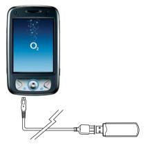
USB On-The-Go (OTG) is a new supplement to the USB 2.0 specification that augments the capability of existing mobile devices and USB peripherals by adding host functionality for connection to USB peripherals.
