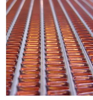
Thanks to strong brazed joints and the reduction of galvanic corrosion at the joints, heat exchangers made by the CuproBraze process are extremely rugged. Their excellent resistance to fatigue and corrosion adds up to a long service life in many appli-
