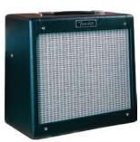
The 15 watt, single-channel Pro Junior is a small all-tube amp, pure and uncomplicated. Features include a single 10" Eminence® speaker, two EL84 output tubes, two 12AX7 preamp tubes, Volume and Tone controls, black textured vinyl covering and silver grille cloth.
