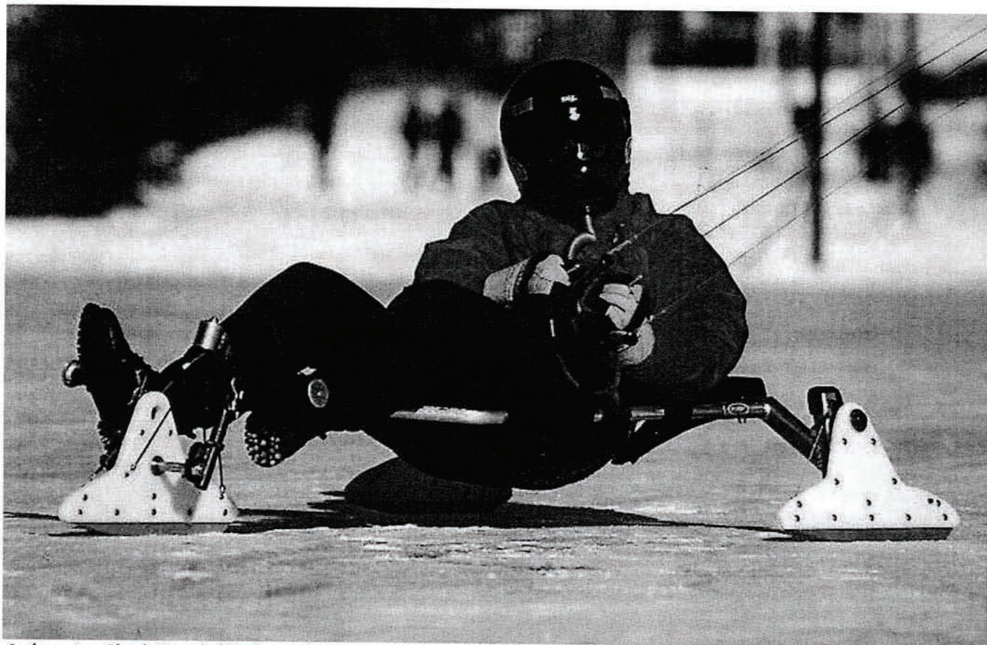
Ice buggying: Claude Gravel of Quebec on the custom made buggy kit he designed for use with Peter Lynn's (model year '97 and up) stiffer and faster buggy frames. Gravel's aluminum buggy frame is shown in photo. Adapting snowmobile polyethylene skis and near frictionless carbide runners used for ice racing on oval tracks, Gravel can travel triple the force of wind and has hit speeds in excess of 60 mph. And it's cold. The temperature was minus 22° C when this photo was taken. Note Gravel's modified boots; they have bolts drilled into the soles for braking on the ice. Braking is also accomplished in the same manner as skiing, using lateral sliding going into the wind.
