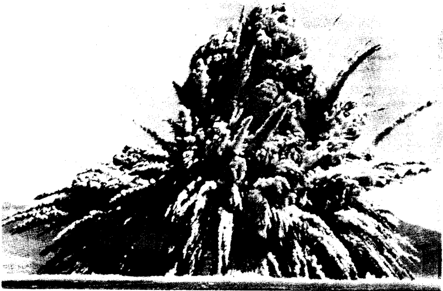
Figure 2.93. Shallow underground burst.
