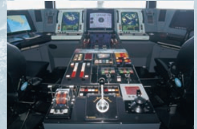
Integrated Bridge Console
