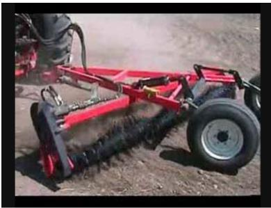
The rock rake concept, along with windrowers and rock-pickers, could be developed into machines for lunar surface stabilization
