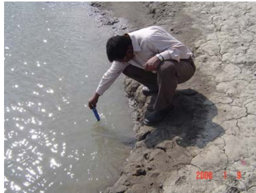
Photo 3.24. Measuring salinity of the water in the Baleswar river
