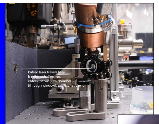
Left: The pulsed laser beam that excites the ion enters through a port at the base of the vacuum chamber.
