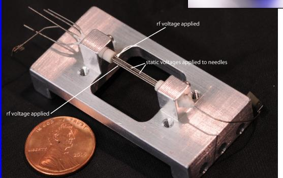
Left: The ion trap outside the vacuum chamber. A total of six electrodes are used to hold the ion in place. Once in position, the ion can be kept in the trap for weeks.
