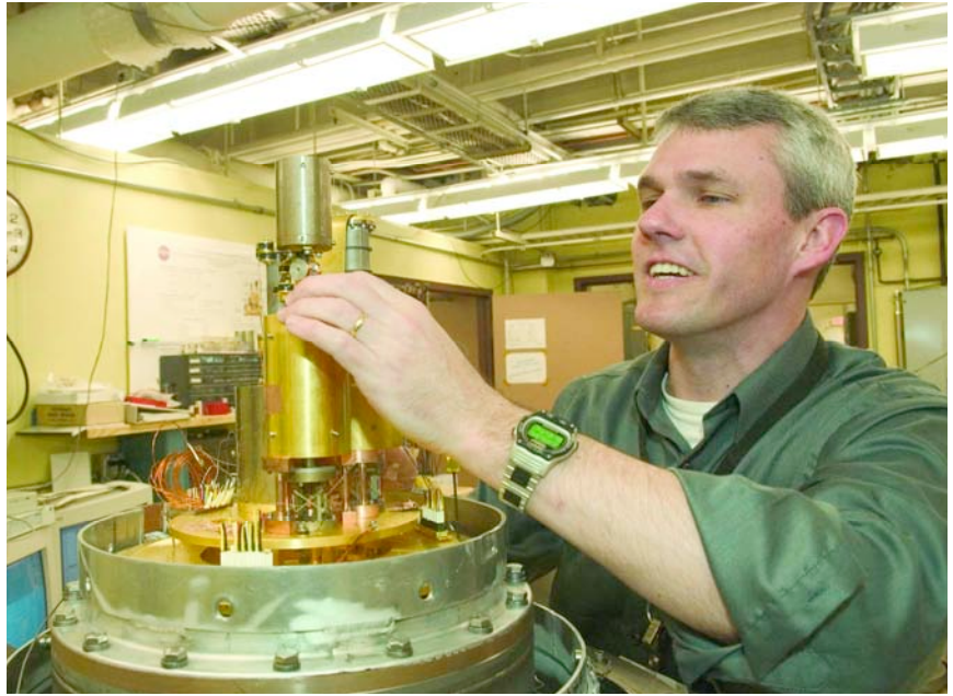
Principal Investigator Peter Shirron, shown here with the Adiabatic Demagnetization Refrigerator (ADR), created three different refrigerants that cool the ADR below the target temperature of 10 mK — important to future far-infrared astronomy missions.
