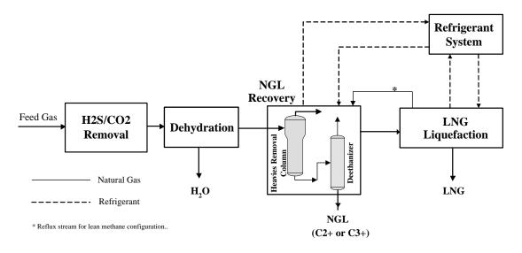
Figure 4 - Block diagram showing the integrated NGL and LNG process
