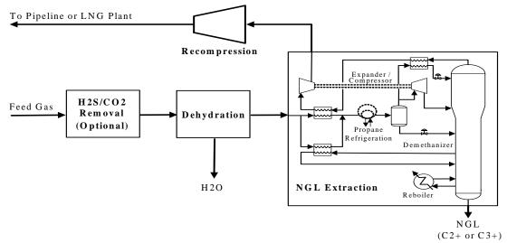
Figure 2 - Block diagram for typical NGL extraction plant
