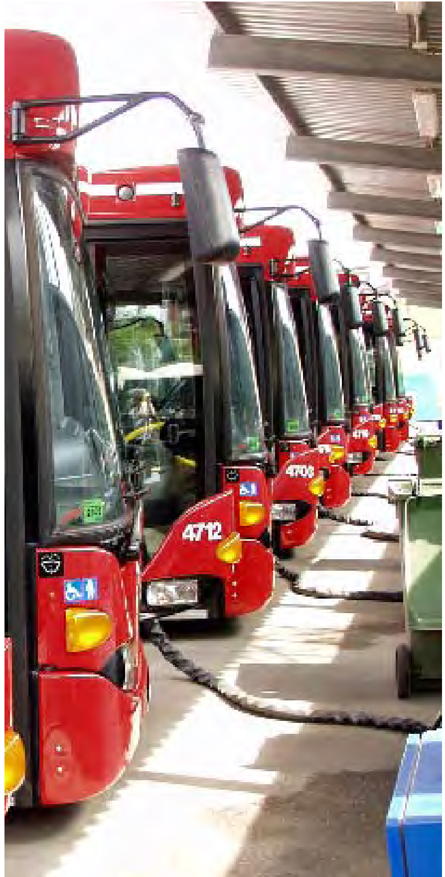
The ethanol buses have contributed to a reduction in SL's diesel consumption by 16 million litres annually.
