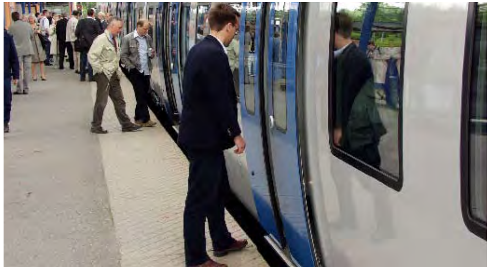
The new commuter train vehicles are articulated and 107 meters long, with an open floor plan throughout. The vehicles have low floor entrances at platform level in all door openings, and a push-out step in the first and last doors. Other features include a low noise level, air conditioning, security cameras, emergency telephones and individual seating.
