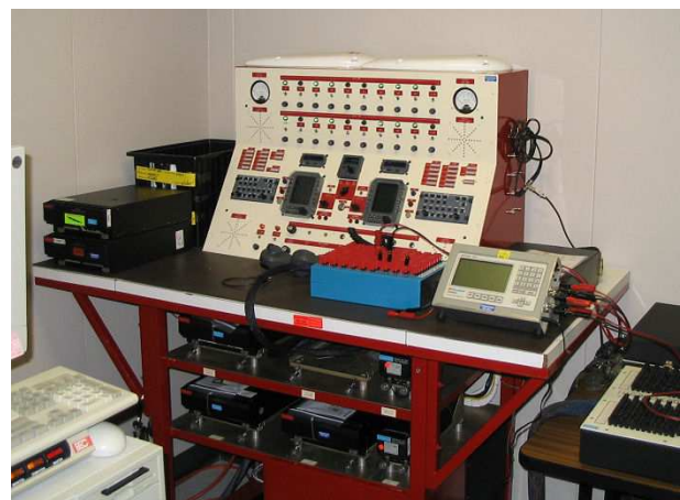
Figure 8. Bench for the Primus II (Radio Navigation)
