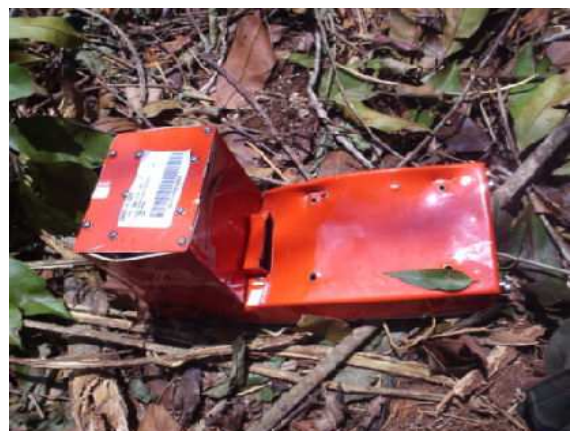
Figure 20: Base of the SSCVR unit, PR-GTD
