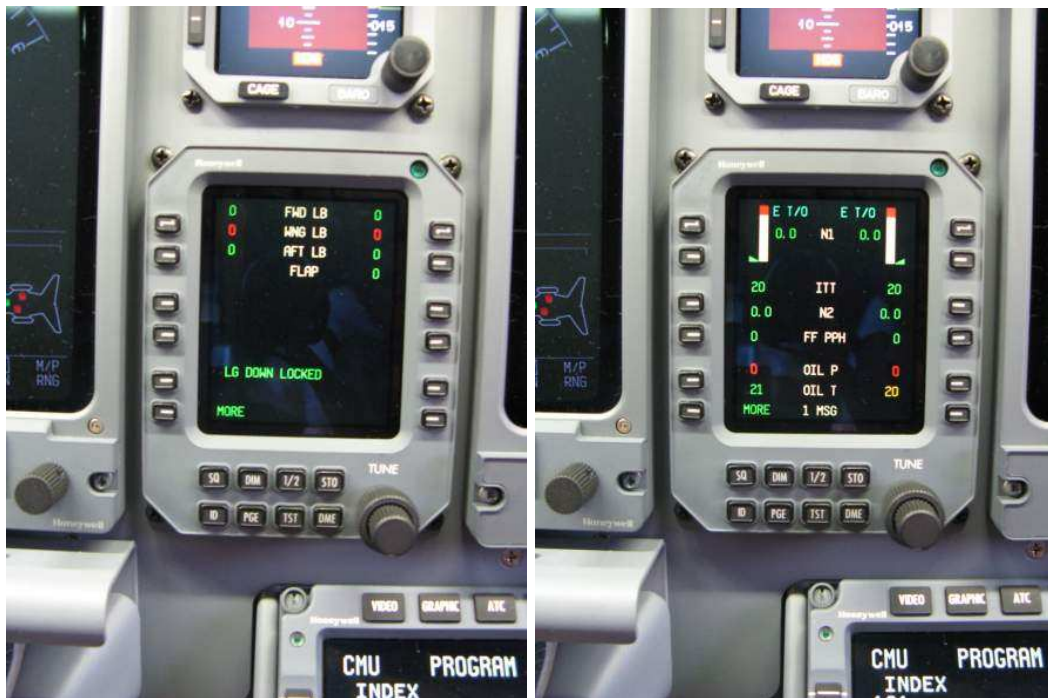
Fig. 69 and 70 (as a back-up, pages with information of the fuel system and engine parameters.
