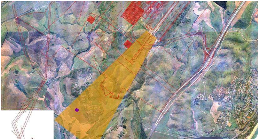
Two dimensional view from above showing runway the 2% obstacle limitation surface and the location of the swallows at the reedbed.
