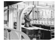
The Bellera "Air Spun" process for milling flour was developed by General Mills in 1960. The new process was less costly and faster than older methods because it drastically reduced the amount of handling and the number of steps necessary to turn wheat into flour.
