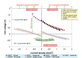
FIGURE 2. Typical Performance Characteristics of a Button-Cell Operated in the Reversible SOFC, SOEC, and SOFEC Modes at 800°C
