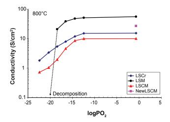
FIGURE 1. Electrical Conductivity of LSCr, LSM and LSCM as a Function of Oxygen Activity at 800°C
