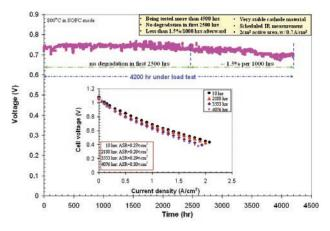
FIGURE 3. 4,200 Hour Long-Term Test (The cell, constructed from a MSRI standard anode tape and deposited with LSCM+SDC-based cathode, was operated in the SOFC mode with a constant load at 800°C. Hydrogen was the fuel and air was the oxidant.)
