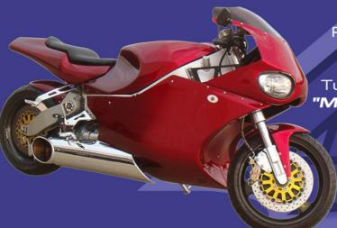
Powered by a Rolls Royce-Allison turbine engine and demonstrating over 320 HP and 425 FT/LBS of torque, the MTT Turbine SUPERBIKE has been named the "Most Powerful Production Motorcycle" by Guinness World Records.
