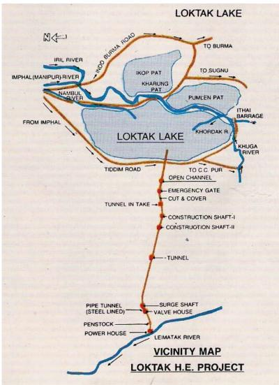
with 5 X 10 m water ways) across the Manipur River is key to maintaining the level at 786.5 meter to ensure steady flow of water from the lake into the narrow Leimatak River which is at the elevation of 312 meters lower than the lake; - thus generating electricity through a well-planned water conducting system.
