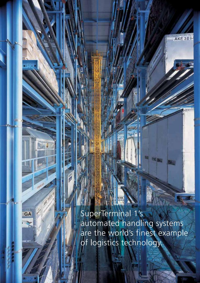
Stretching from the eastern to western perimeters, and rising to the same height as the terminal building, the Container Storage System (CSS) is fully automated and provides a direct and sheltered interface with the airside, allowing cargo units and pallets to move swiftly between the system and the tarmac. In addition, the CSS offers:
