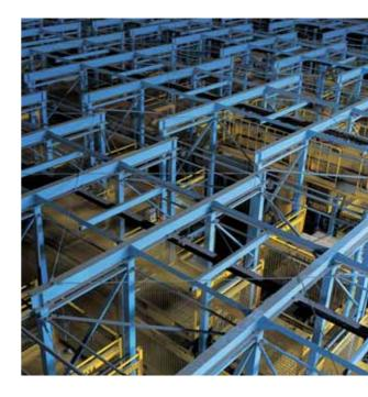
The Box Storage System (BSS) is another example of advanced logistics technology. Located at the heart of the terminal building, the BSS automates the movement of bulk cargo in the terminal building without the need for human intervention.
