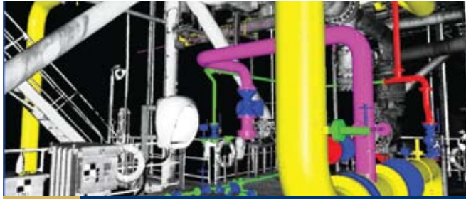
FIG. 3 CAD model "back projected" into a laser image of a facility.
