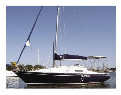
utilizing the two solar panels as a bimini creates plenty of shade for the cabin.
