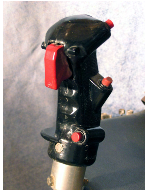
UH-1 Cobra Joy Stick provides vehicle vector control and four channels of electrical control.
