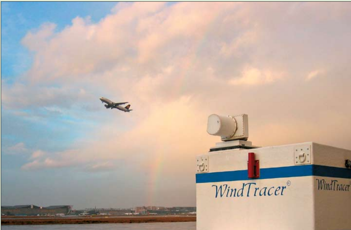
A Doppler lidar (light detection and ranging) system developed to detect dangerous wind conditions at airports, WindTracer can also be used by wind farm developers to select locations with the strongest and most consistent winds.
