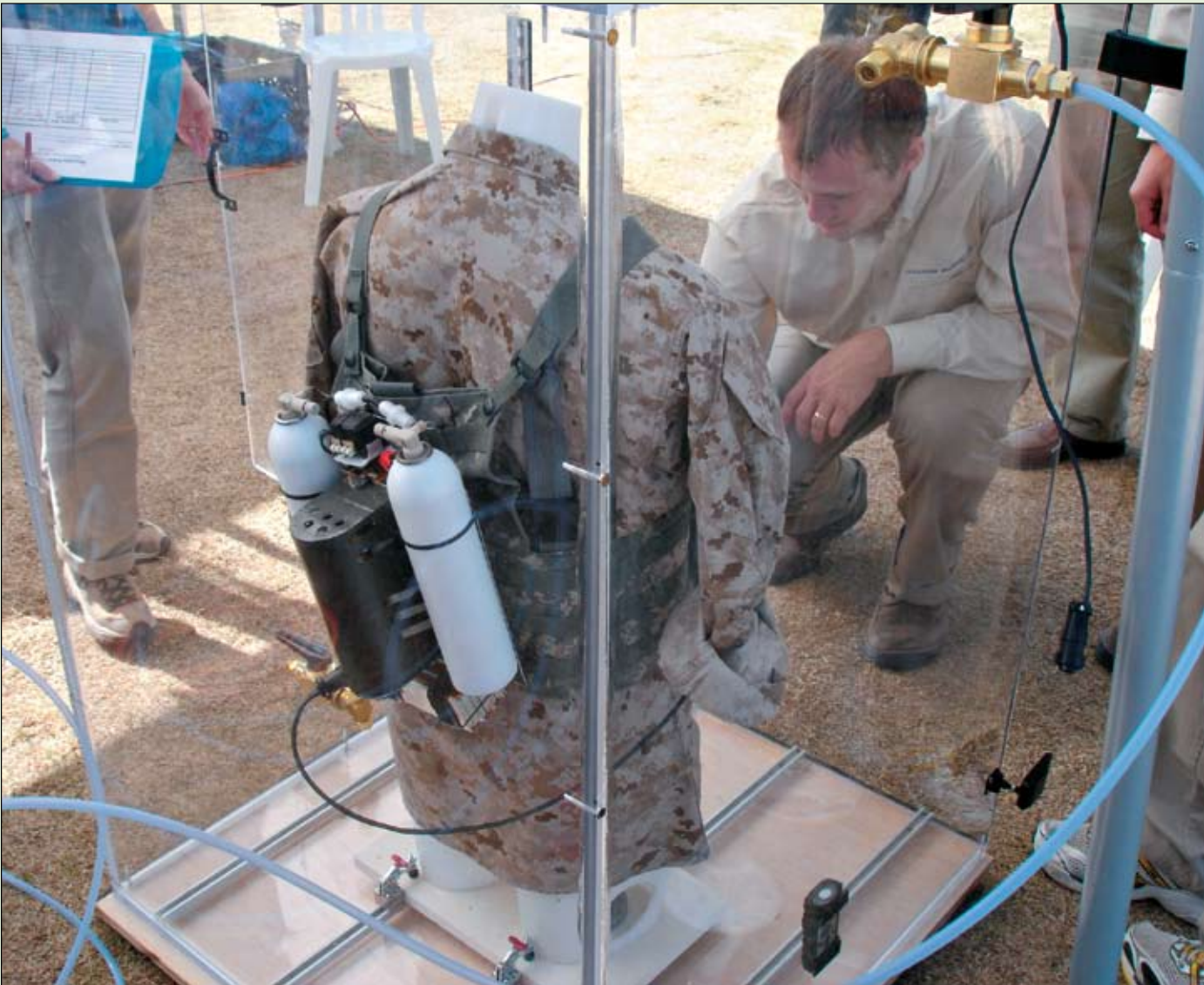
The Power Management team at Missiles and Fire Control has developed several portable battery products for effective energy storage. Here, Senior Electrical Engineer David Hoelscher checks out a power pack that can be worn by soldiers.
