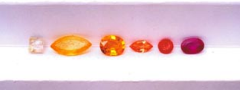
Beryllium diffusion treated corundum. © H.A. Hänni, SSEF 2003
