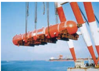
Heavy-wall pressure vessel for oil refining
