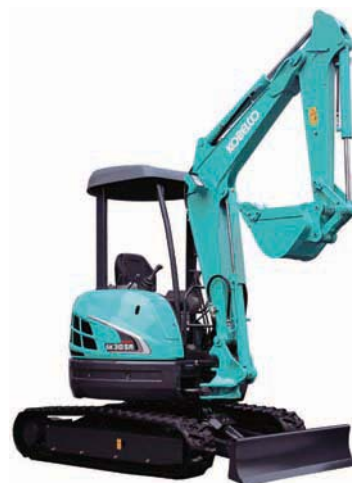
Excavator with short tail swing radius
