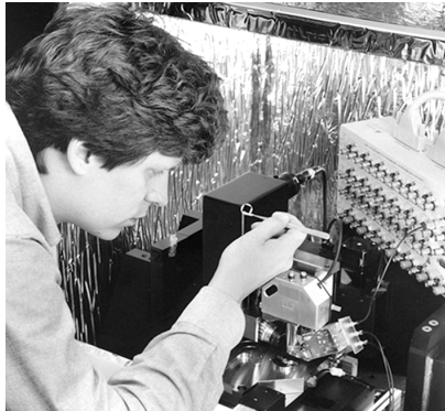
Loading a sample into the scanning capacitance microscope.
