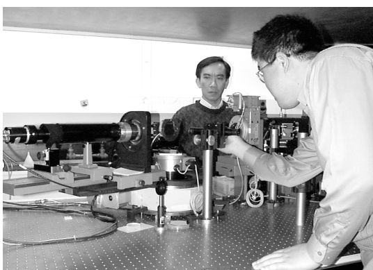
SED researchers align sample on custom-built high-accuracy spectroscopic ellipsometer.
