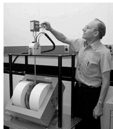
The Materials and Technology Group's Bob Thurber connecting cables to the sample holder for a Hall effect measurement.
