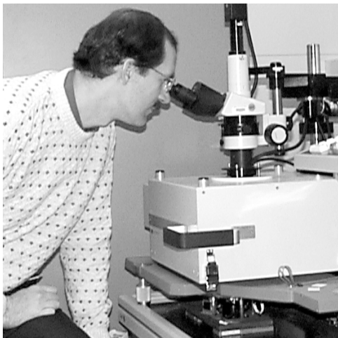
Aligning probe card to silicon substrate under test.
