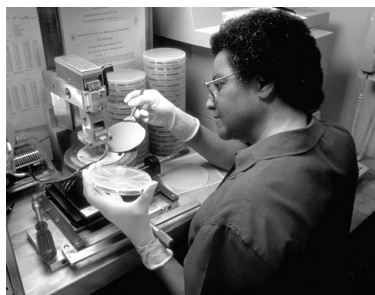
Donnie Ricks of the Thin-Film Process Metrology Project mounting a silicon wafer on the resistivity instrument stage prior to taking measurements for SRM certification.
