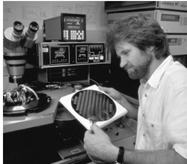
Test wafer being loaded on wafer probe for long-term dielectric testing.
