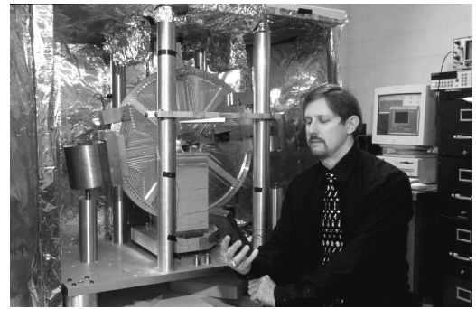
Richard Steiner working with the test balance used for studies of knife-edge hysteresis.
