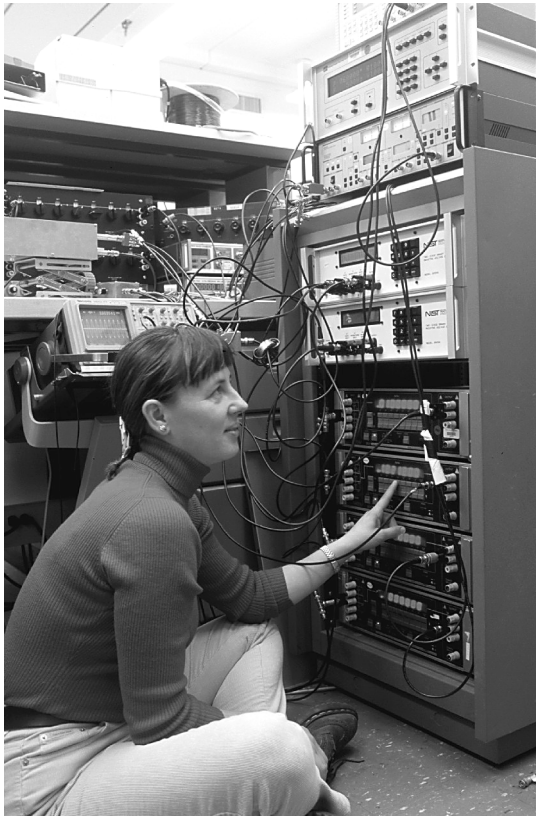
Guest Researcher Svetlana Avramov-Zamurovic adjusting the new wideband capacitance scaling bridge.
