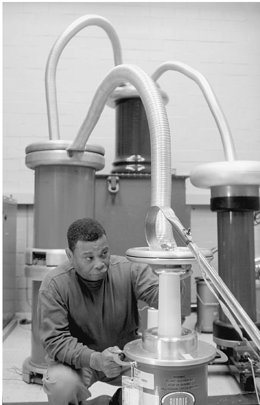
James Pitt connecting a capacitive high voltage divider to the ac high voltage power supply.
