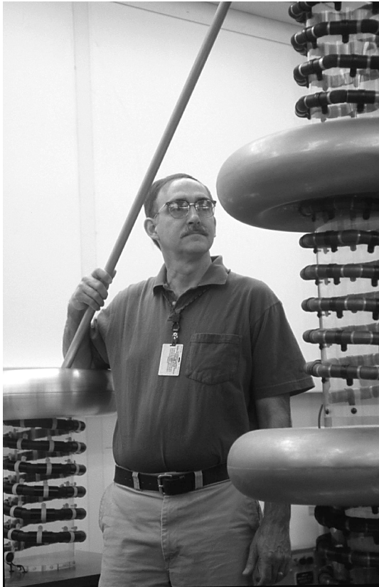
Ken Stricklett connects a high voltage dc divider to the NIST reference divider and high voltage power supply.
