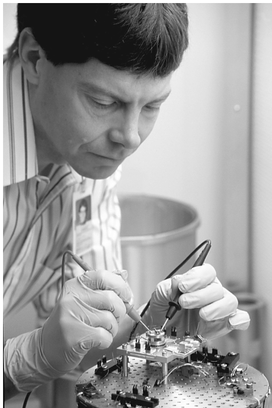
Tom Lipe installing new transition edge sensor (TES) chip in cryogenic-based thermal transfer standard system.
