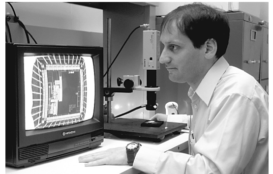
David Bergman examining the new low-thermal-error ASIC sampling comparator.
