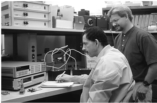
Dean Jarrett (NIST) (R) assists Harold Sanchez (ICE, Costa Rica) in the development and evaluation of a measurement technique to be used in Costa Rica for the calibration 10 G \Omega and 100 G \Omega high resistance standards.
