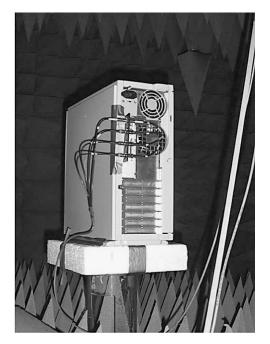
Measuring the radiation characteristics of a typical device-under-test in the NIST anechoic chamber.
