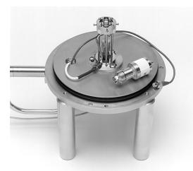
2.4 mm microwave calorimeter and detector
