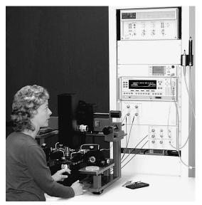
Dr. Kate Remley performs large-signal measurements of an RF power amplifier using the Nonlinear Network Measurement System
