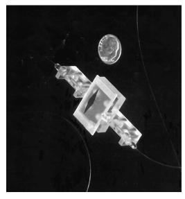
Integrated resistively-tapered dipole and electromagnetic modulator
