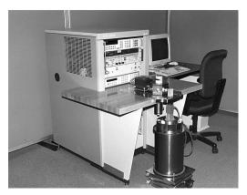
Noise figure radiometer and cryogenic standard
