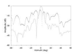
Antenna pattern (solid line) and the result of a simulated measurement (dashed line) where random probe position errors on the order of a wavelength have been introduced (normal measurement spacing is  $\frac{1}{2}$  wavelength). NIST software permits accurate, efficient recovery of the original pattern. The corrected result is not distinguishable from the original on the scale of this plot.
