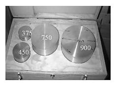
The basic cylinder set used to calibrate static RCS measurement systems in the frequency range of 2-18 GHz. The cylinders are made of aluminum, and are manufactured to a tolerance of  $\pm 0.0127$  cm.
