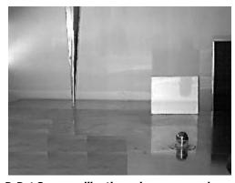
D-Dot Sensor calibration using a cone and ground plane standard-field generation system.
