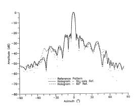
Comparison of the far field as determined by conventional near-field methods (dotted line) and from thermal imaged holograms (dashed and solid lines).
