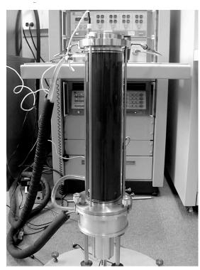
**Cylindrical Cavity Resonator**
