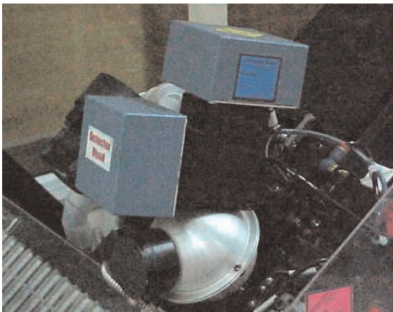
Figure 13. Optical detector assembly used for amber, red-orange and red SuperFlux and SnapLED emitters. Note the small integrating sphere in the lower area of the picture. The two optical detectors (gray rectangular boxes) are mounted to the integrating sphere with a beam splitter (black cube).
