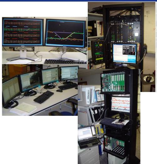
Communication-based on-board and wayside signaling equipment from four suppliers interoperable with each other
