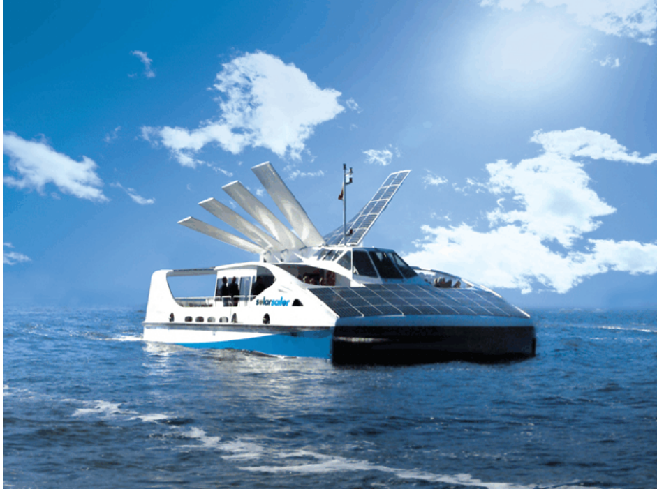
Figure 11. Solar Sailor Hybrid-Powered Ferry Boat
