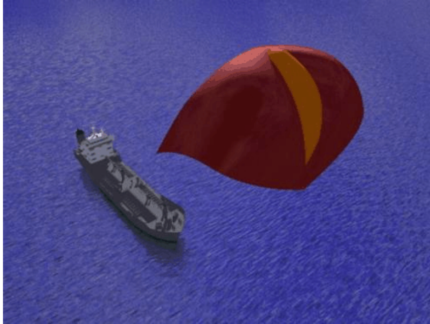
Figure 8. KiteShip Concept Applied to Commercial Cargo Ship
