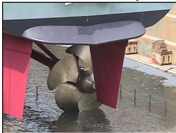
Figure 3. Stern Flap on DDG-51 Class Destroyer
