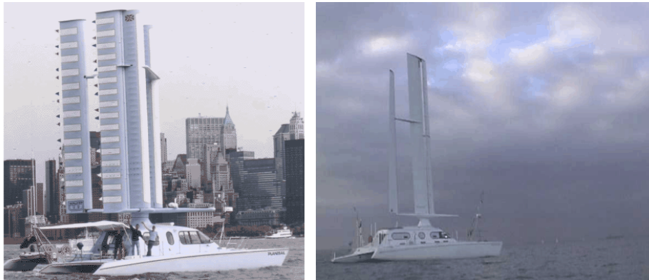
Figure 6. Pleasure Craft Equipped with Walker Wingsails
