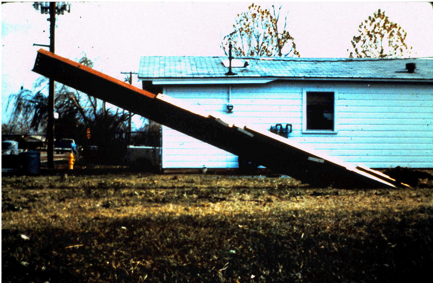
One of several 700 pound I-beams stuck deep into the ground by the tornado. (Photo courtesy of Ernest Ethridge)
