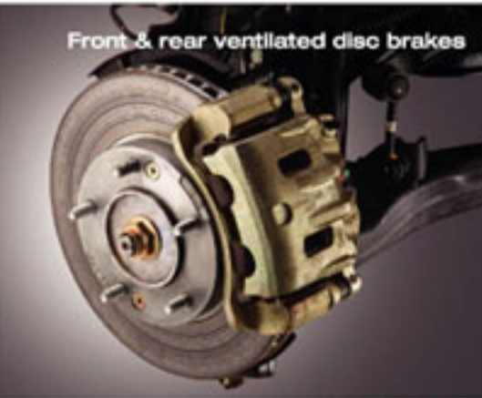
Front & rear ventilated disc brakes
