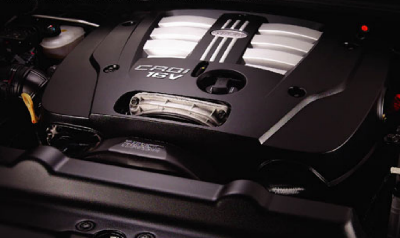
CRDi (Common Rail Direct Injection) Turbo Intercooled 2.5-litre engine
