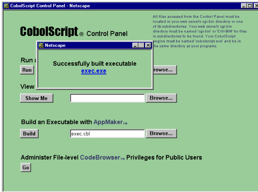
Figure 9.6— Creating an executable with AppMaker from the Control Panel.
