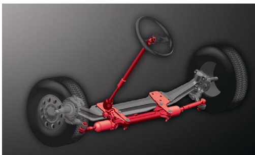
Freightliner's industry-first rack and pinion steering system , available with spring or front air suspensions, is responsive and provides tight control. (Available on 120 model only.)
