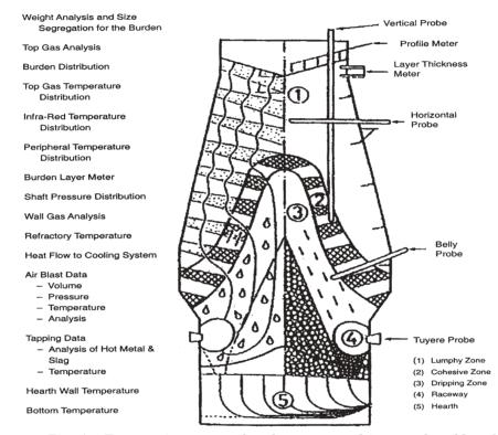
Fig. 4 : Features incorporated and sensors used in a modern blast furnace
