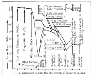
Fig. 3 : Oxygen to iron ratio during iron and steelmaking
