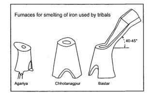
Fig. 1 : Remnants of primitive iron making furnaces
