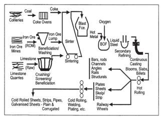
Fig. 2 : Present day integrated iron and steel works
