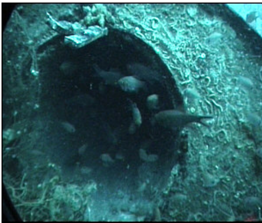
Figure 51: Detail of damage to the upper torpedo tube.
