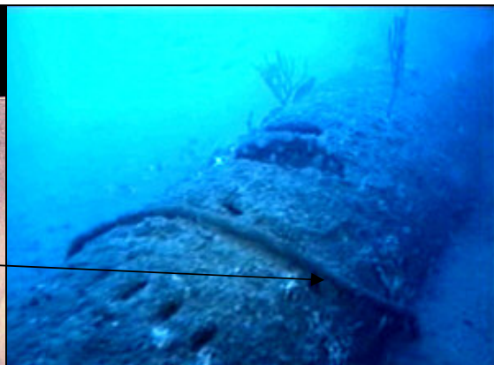
Figure 31: Detail of fishing net line wrapped around the M24 hull at aft tail section. Photo: Heritage Office/Royal Australian Navy.
