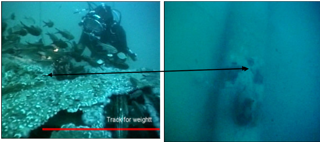
Figure 58: Detail of corrosion opening on port hull, aft.
