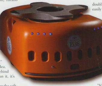
The robots in Staples' facility charge their own batteries and require little maintenance.
