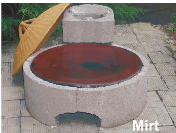
“Mirt” Enjera Closed Stove efficiency b/n 25-35% during operation (EREDPC)
