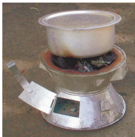
“Laketch” Charcoal Saving Stove” in operation (EREDPC)
