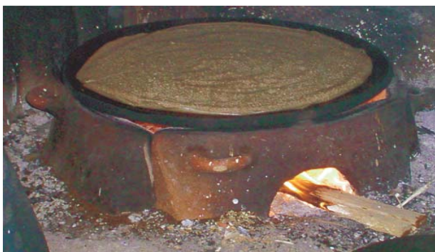
“Gounzie” (closed Enjera Stove) efficiency about 47% during test. (EREDPC)
