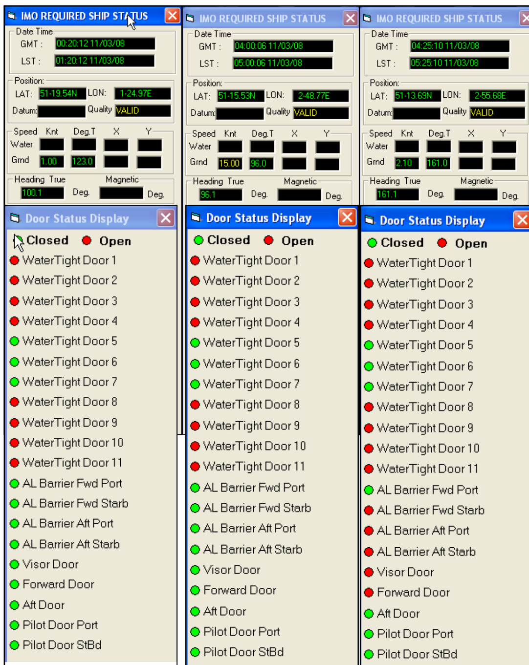
Extract of VDR data showing the status of the watertight doors on the vessel's previous passage
