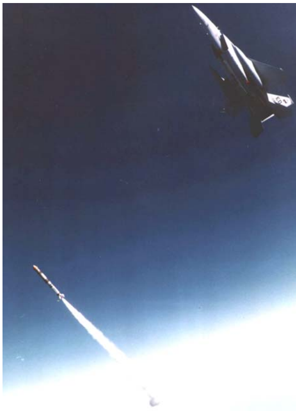
Left: The Air-launched Antisatellite missile is released from its F-15 launching aircraft and its motor is ignited. At a certain point in its trajectory, the missile released a miniature homing vehicle which destroyed the satellite by impact. Below: A cutaway view of the ASAT's miniature homing vehicle. The rockets were mounted in an outer ring around the vehicle, and the infrared seeker assembly was in the center.
