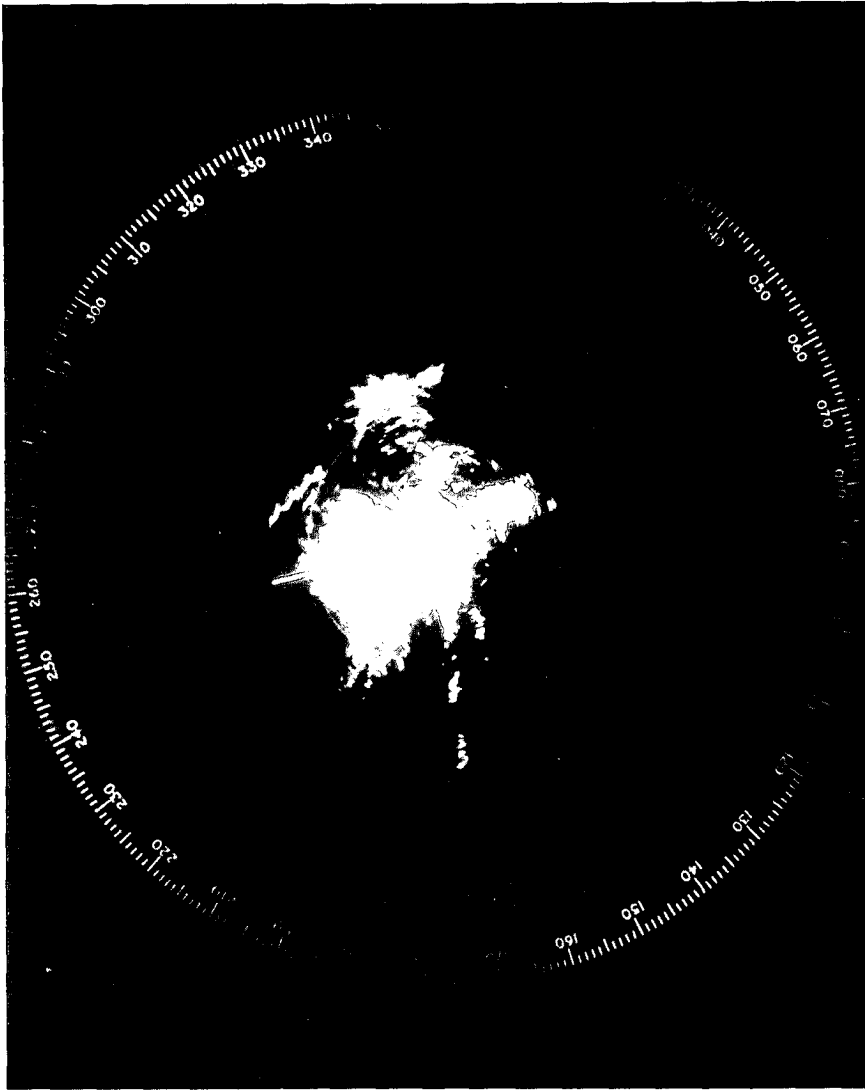
Figure 37. Radar picture of Typhoon 'Irma' taken at the Royal Observatory at 8.00 a.m. on December 2, 1974 (Range markers at 40 n mile intervals).
