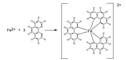
Once a colored complex is formed, the wavelength of light which is most strongly absorbed is found by measuring the absorbance at various wavelengths between 400 - 600 nm. After the most suitable wavelength is determined, a series of iron standards is measured at this wavelength and a calibration plot of absorbance vs. concentration is prepared. The absorbance of the unknown sample is measured and the calibration curve is used to calculate the concentration of iron in the sample.
