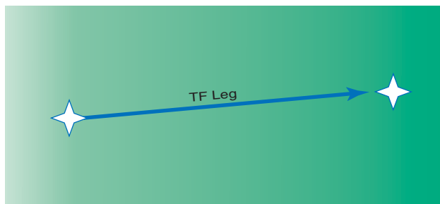
Figure A-7. Path/Terminator. A Path/Terminator value of a TF leg indicates a great circle track directly from one fix to the next.
