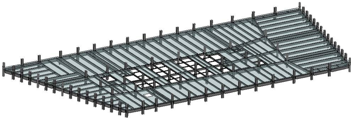
Figure 3-29. Standard tenant floor structural framing and slab model (Floors 8 through 20 and 24 through 45)
