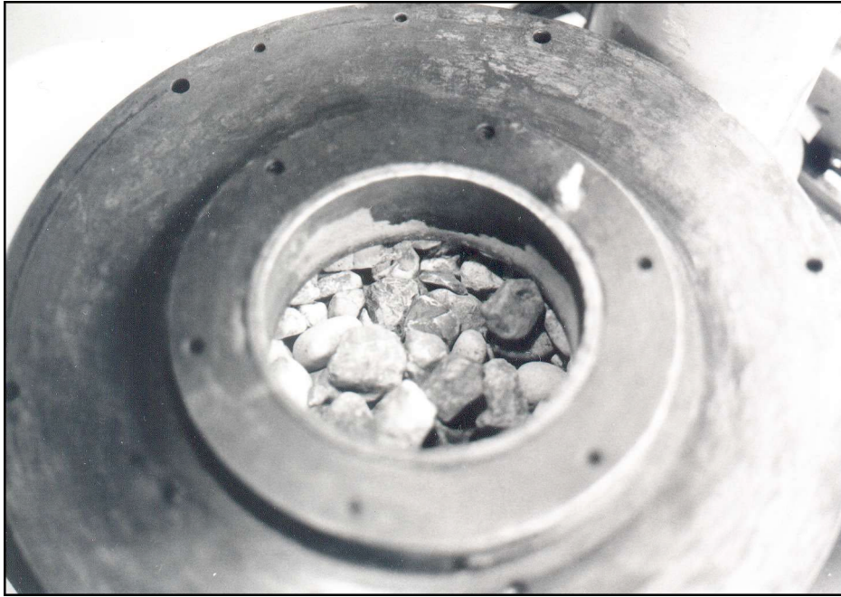
Picture No. 2 is looking down into the 6" diameter grinding chamber.
