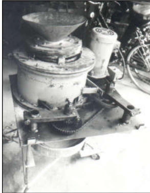
Picture No. 1 is the complete grinder with dust collection pan, top head and hopper.
