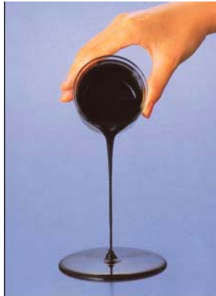
Figure 9 Pouring a CWF at room temperature [32]
