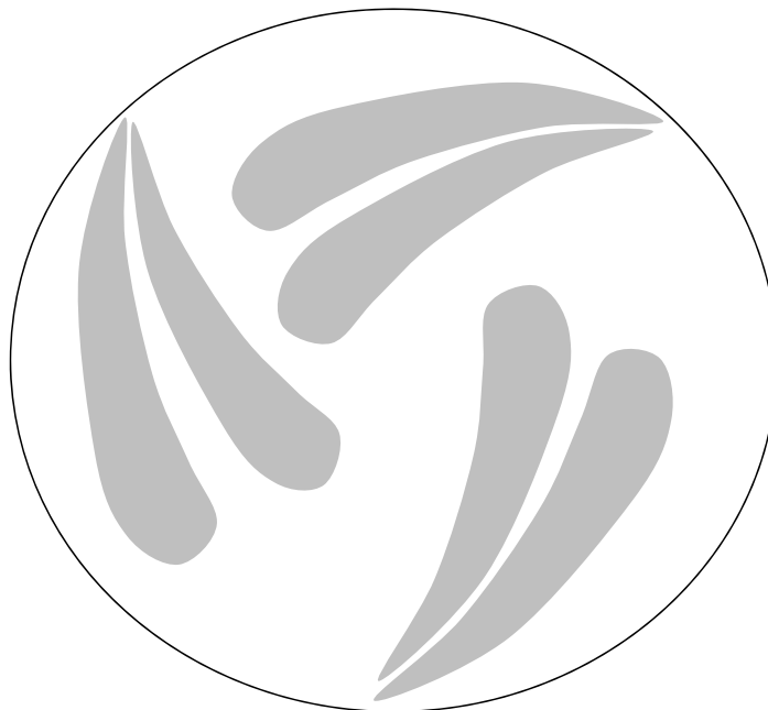
Figure 18 Typical injection spray patterns for a large 2-stroke engine using high swirl and peripheral injectors
