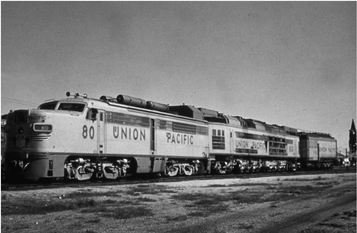
Figure 12 Union Pacific 4,500 hp (UP80 class) coal turbine locomotive set with coal tender at the rear circa 1960 [38]
