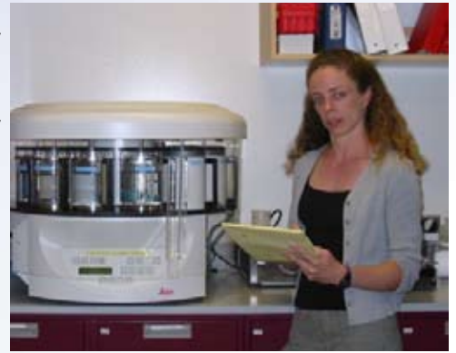
Dr. Marta de Maintenon prepares invertebrate tissue samples for microtome preparation of slides using an automatic tissue processor. The Analytical Facility includes a freeze dryer, autoclave, an E-Pure Reagent Water system and other sample preparation equipment.
