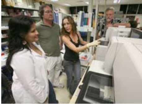
Tatiane Varys, Donald Price, Anne Veillet, and Cam Muir examine the Beckman Coulter CEQ 8000 in the Hilo Core Genetics Facility. This is the main instrument used in sequencing and genotyping in the lab.
