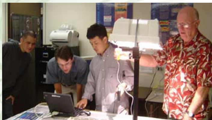
Dr. Kassis, W.M. Keck Observatory, and Dr. Park, UHH, measuring the relative throughput of optical elements in the overhead projectors used at W.M. Keck Observatory as flat fielding lamps for MOSFIRE, a near-IR (~0.97-2.45 \mu\text{m} ) spectrograph for the Cassegrain focus of scientific instrument Keck-I.
