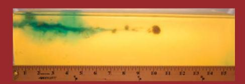
45Auto 165gr PowR'Ball Glock Model 21 4.6" barrel 92% weight retention
